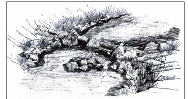
C | Drop structure using indigenous log construction.
